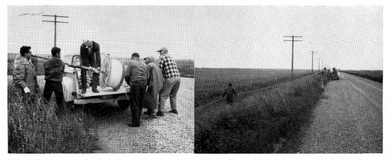
FOR 20 MILES along the Canadian prairie, Sandians strung lines and placed 18 sensors to detect airblast waves from a 500-ton high-explosive experiment. Six camper-trailers housed the recording
